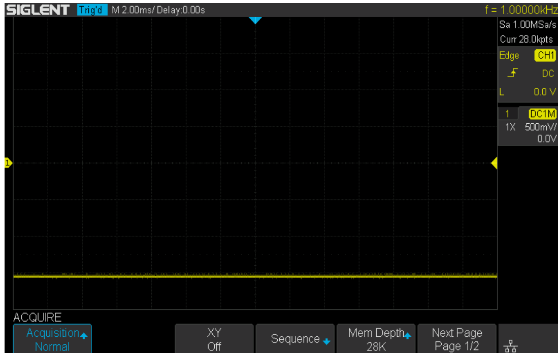
Figure 16 Pulse With 0.01% Duty, Normal Mode
